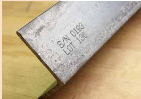
Deep mark on structural steel
