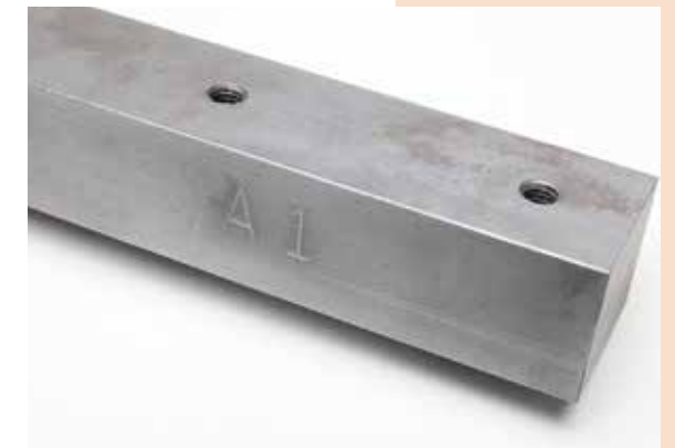
Marking on hardened material HRC62
