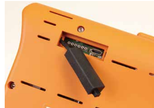
USB connector for PM Win Software. (standard equipped)
